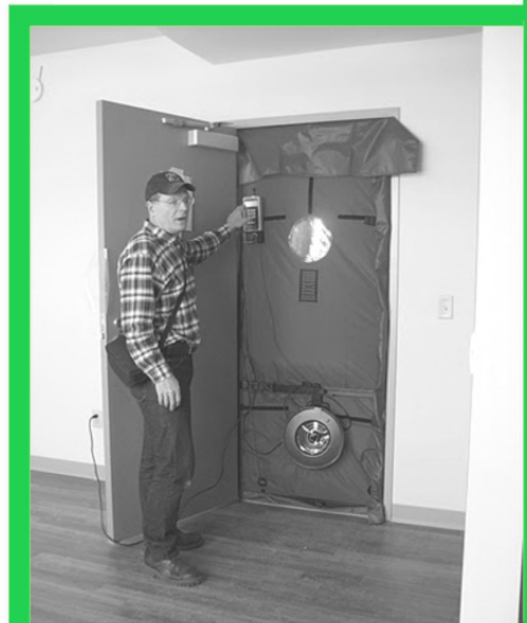
Blower Door Test, Performed During Energy Audit
